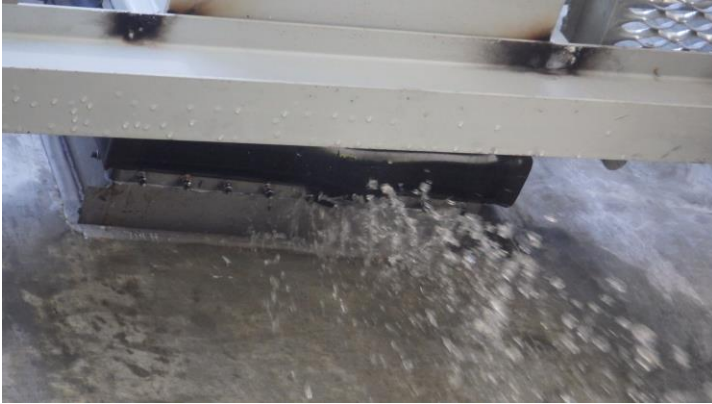
Photo 2. Closer photo of expansion joint leak between the PDW and the transport flume.
